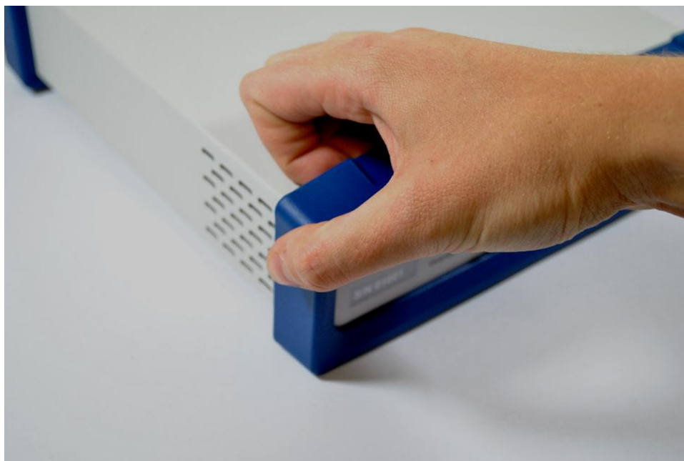
Figure 3-4 Removing the Front Bezel
