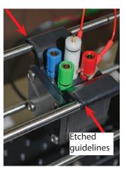
To firmly attach the cell to the rails, you may add two clips at diagonal corners. Tighten the clips with an 0.035" Allen key.
