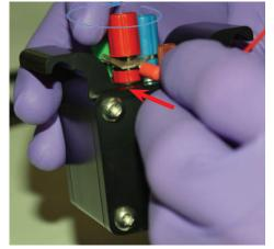
Insert the Pt wire into the adapter.
