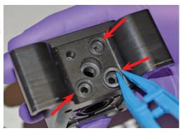
Over the O-rings, screw in the three colored electrode adapters.
