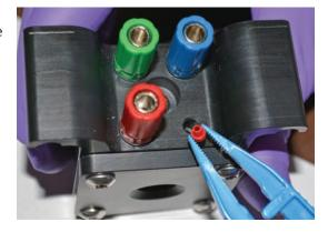
Screw the VacuTight™ fitting into the hole with the ferrule.
