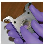
Place the front plate onto the sapphire window.
