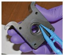
Place the optical sapphire window onto the O-ring.
