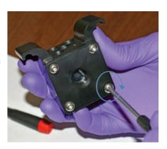
Assemble the rear side of the cell body.
