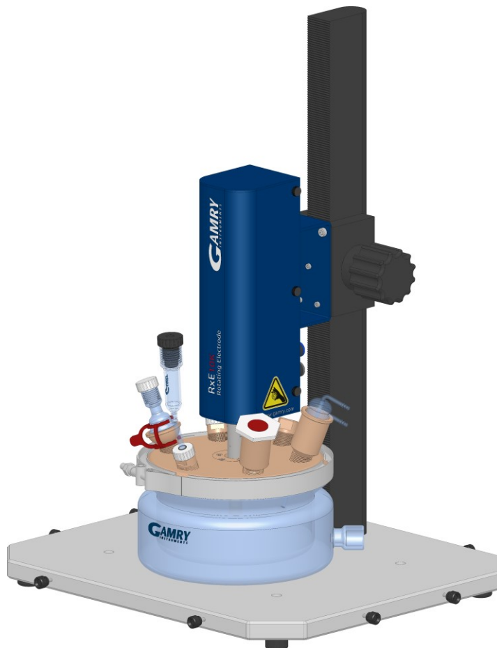
Figure 2.12 RxE 10k rotator in use with a 1L RCE Cell.
